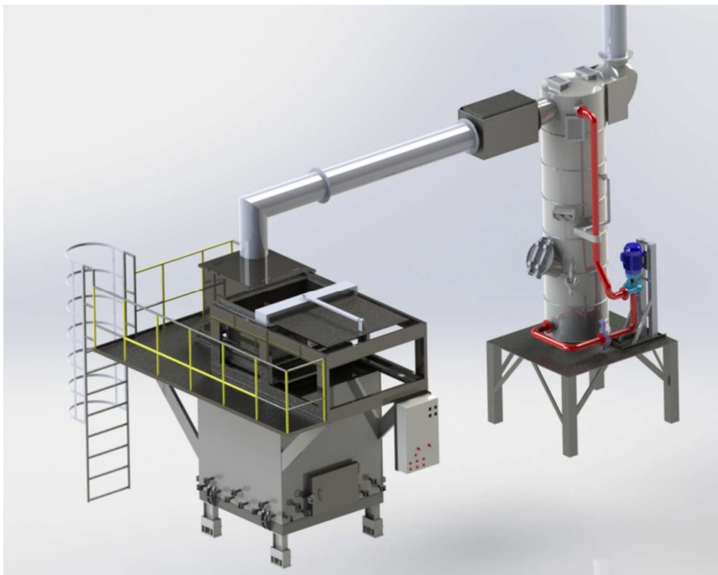
Figure 2 – Schematic of the OXYCLEAN system with the combustion chamber on the left and the fume treatment (Venturi scrubber) on the right.
